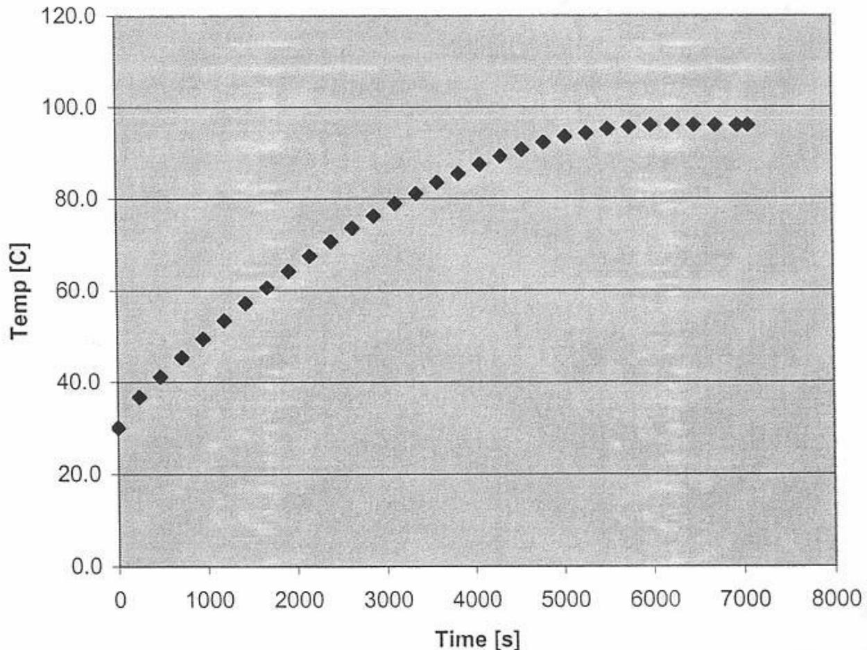
Comparing the two graphs above, we find that the Solar CookKit performed very well, comparable to the Funnel Cooker. We should note that in both cases, we used a canning jar (pressurised) supported by a wire stand. We found that the wire stand improves the performance of the Solar CookKit significantly and hope that this support stand will be used in countries where the Solar CookKit is in use.
