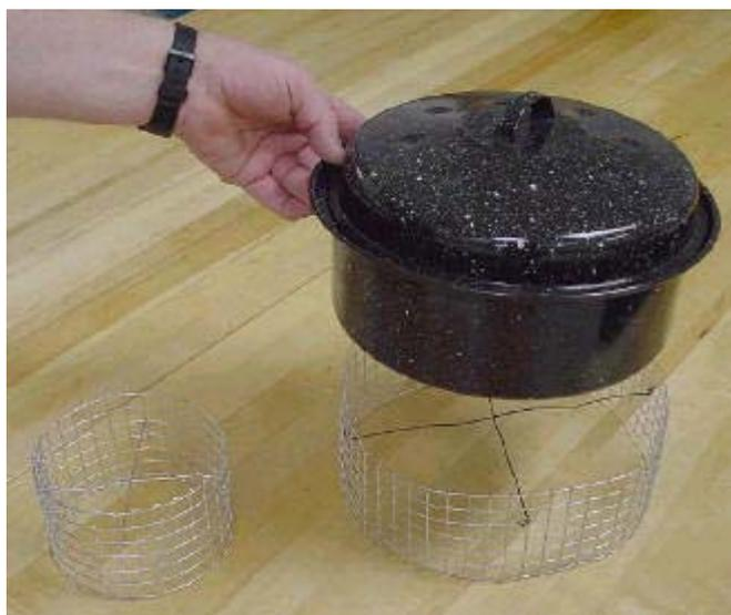
The third main area of focus is in the cooking containers used. The present cooking vessel for the Solar Funnel Cooker is a black-painted canning jar. This method is also tedious and awkward. The canning jars can be hard to clean, and they can break. Design changes are tested that would allow people to use their own cookware. This too would make the cooker more convenient to use.
